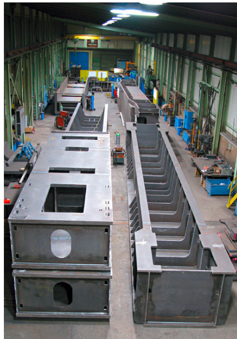
JUNG production hall: various traverses (length: 15 - 20 m, weight: approx. 50 - 75 t)
