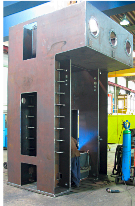
Machine stand (length: 6.8 m, width: 4.2 m, height: 3.5 m, weight: approx. 48 t)
