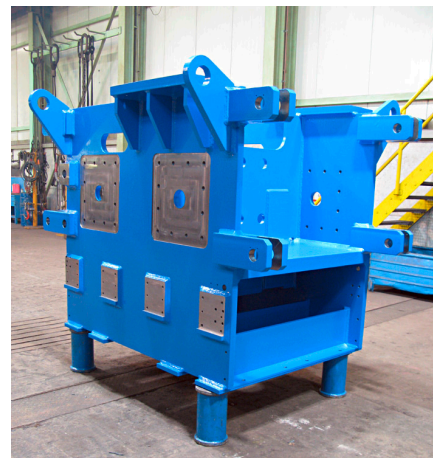
Frame for sheet metal forming (length: 3 m, width: 2 m, height: 2.5 m, weight: approx. 7 t)
