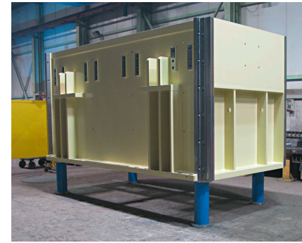
Press ram for a 1,000 t double-column press (length: 5.5 m, width: 2.9 m, height: 2.7 m, weight: approx. 56 t)
