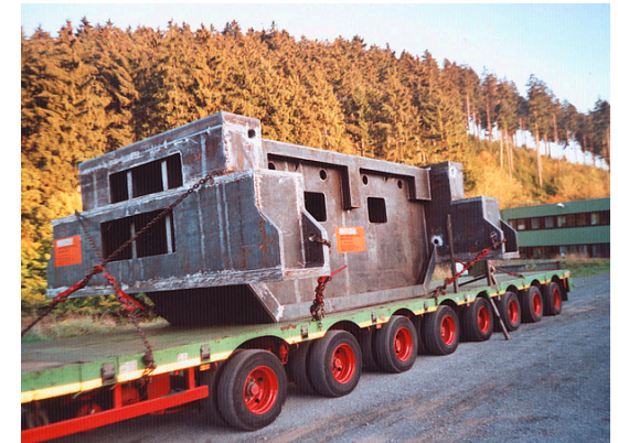
Transport of a press table (length: 6.2 m, width: 4.65 m, height: 2.4 m, weight: approx. 85 t)
