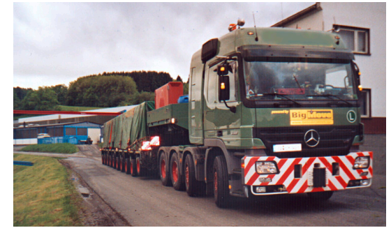
Transport of a press frame (length: 20 m, width: 3 m, height: 2.8 m, weight: approx. 86 t)
