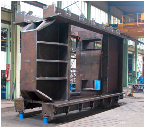
Double column press (length: 6 m, width: 4.2 m, height: 2.2 m, weight: approx. 53 t)
