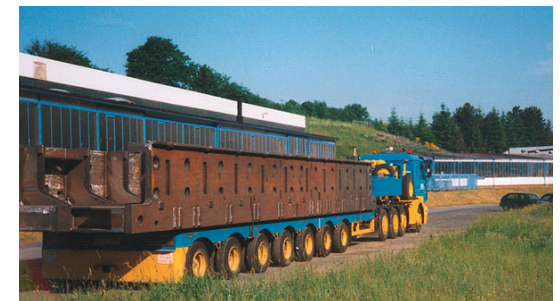
Transport of a traverse (length: 15 m, width: 2.6 m, height: 1.8 m, weight: approx. 76 t)
